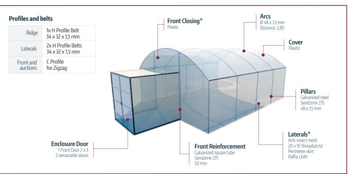
\* Note: Front and side walls will be buried for its lower fixing.
